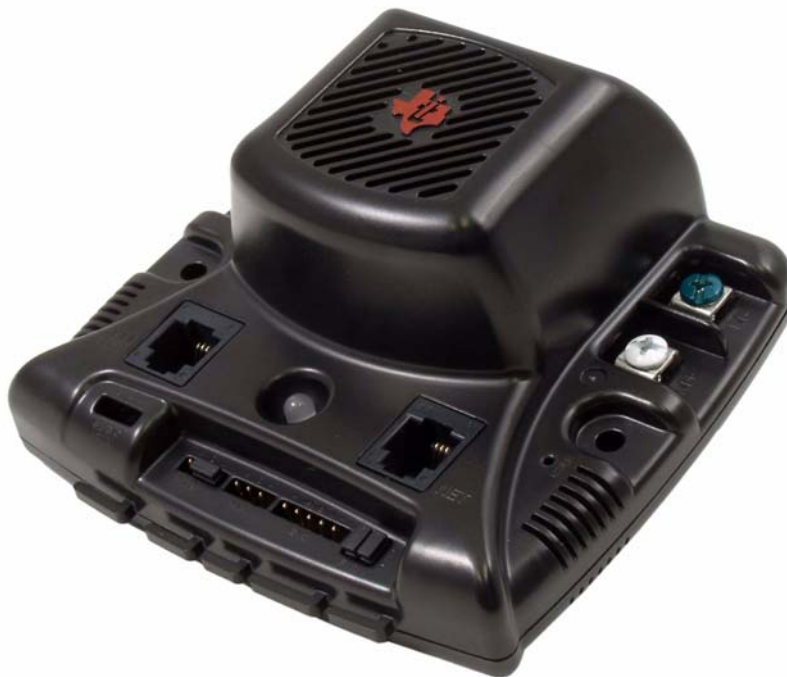
Figure 1-1. Next Generation Brushed DC Motor Control Module, MDL-BDC24
